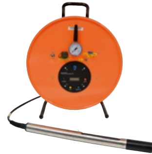
BGK3/7 | Borehole Geophone
