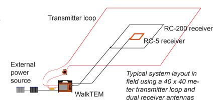
An external power source, a car battery or similar, can be connected with the supplied external power cable. This will provide more power and thus enables more hours of survey.
