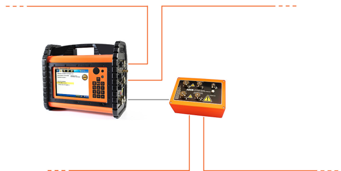
The Terrameter LS system can be expanded using optional relay switches (ES10-64), each adding up to 64 electrodes to the array.
